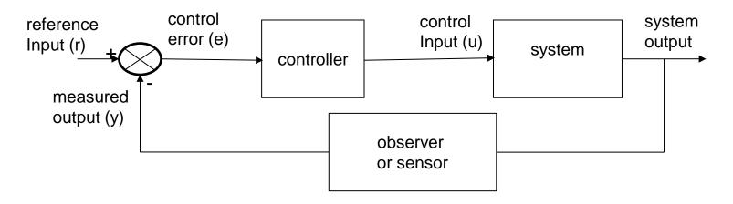
Controller aims to maintain the difference between the reference input (e.g., performance targets as desired values) and the measured output (e.g., measured performance metrics), in spite of disturbance, noise, or attack that are not under control
